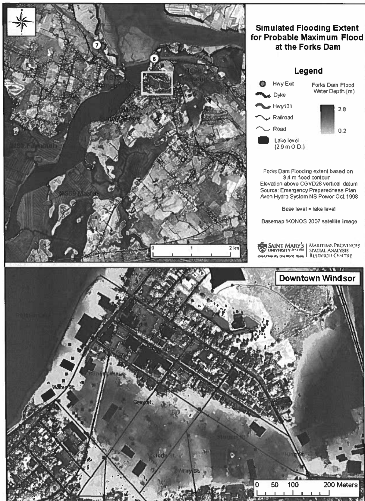
Figure 10: Simulated flood event for a probable maximum flood at the Forks Dam depicted damage to the Town of Windsor.
